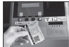
and CTfastrak buses issue 2-Hour Passes (transfers) and All-Day passes using bar-code reading technology rather than magnetically encoded stripe technology. The bar code is printed on the front of the pass. Scan the bar code on the window with the red light on the fare box – a tone will sound indicating acceptance.
